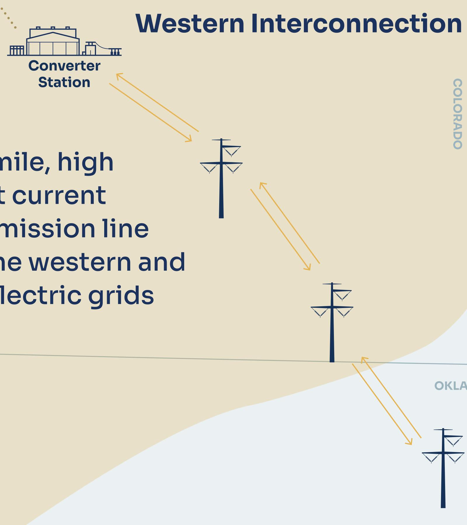
Up to a 300-mile, high voltage direct current (HVDC) transmission line connecting the western and eastern U.S. electric grids
